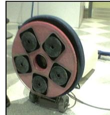
KM 175 fitted with a diamond disc holder & diamond honing discs
