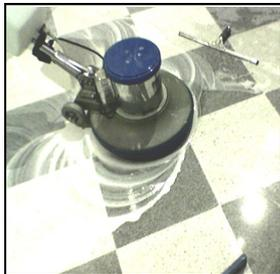
KM 175 is extremely efficient at diamond disc honing, crystallization and powder polishing all types of marble and terrazzo floors due to its ideal weight and speed
