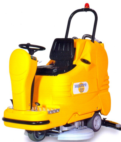
Adiatek Sapphire 85, battery 36V 85cm cleaning width, 115cm suction 110/120 L Solution/Waste tanks
